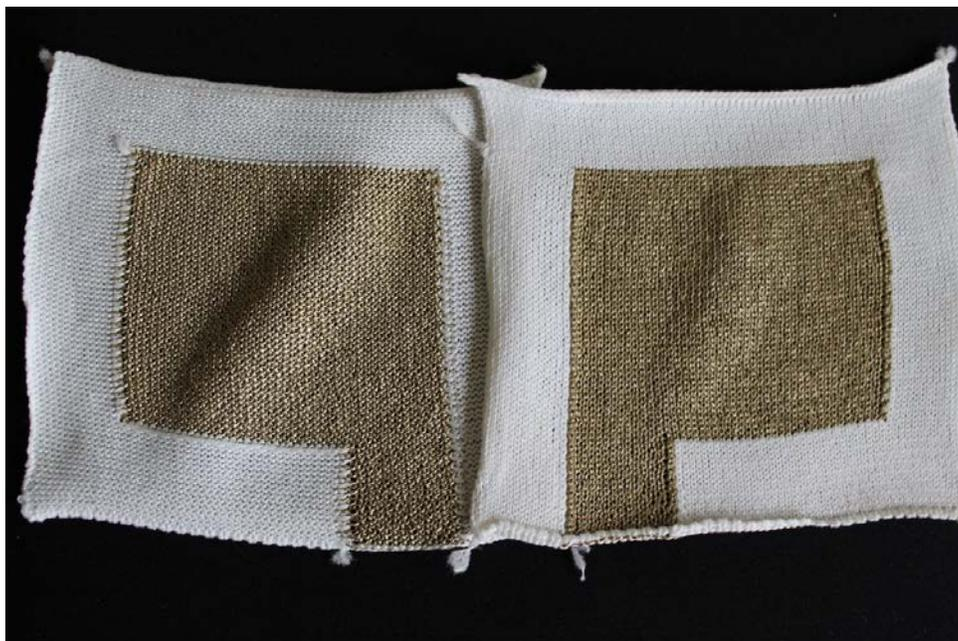
*Figure 1: Knitted conductive panels made from silver coated yarn*
