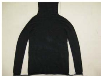
*The garment as it leaves the knitting machine complete with draw thread*
